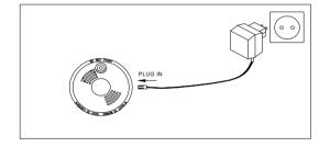
the unit is connecting to power. Depress the test button about 5-10 seconds until the alarm sounds to ensure the alarm is operating mode.
