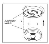
Install the mounting bracket on the wall. Alignment marks of the mounting bracket and Plug the power connector into the gas alarm, the green LED illuminates to indicate the gas alarm should be lined up for power connector plug in. Twist the alarm clockwise until it locks in place.
